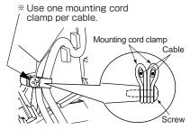
Fasten the clamps together with a screw.
