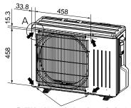
Drill the lower holes through the front paneland the base.
